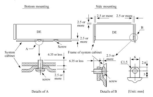
Figure 4.4 Mounting frame structure
